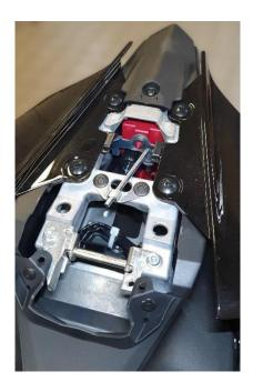
Modification of the chain protector/rear mudguard (in order to facilitate operations of rear wheel changes, it is permissible to cut the plastic chain protection up to the red mark as below), however, it is prohibited to remove the entire mudguard:
